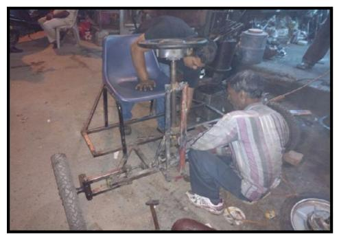
Figure: Workers helping in Adjusting Steering Column.
