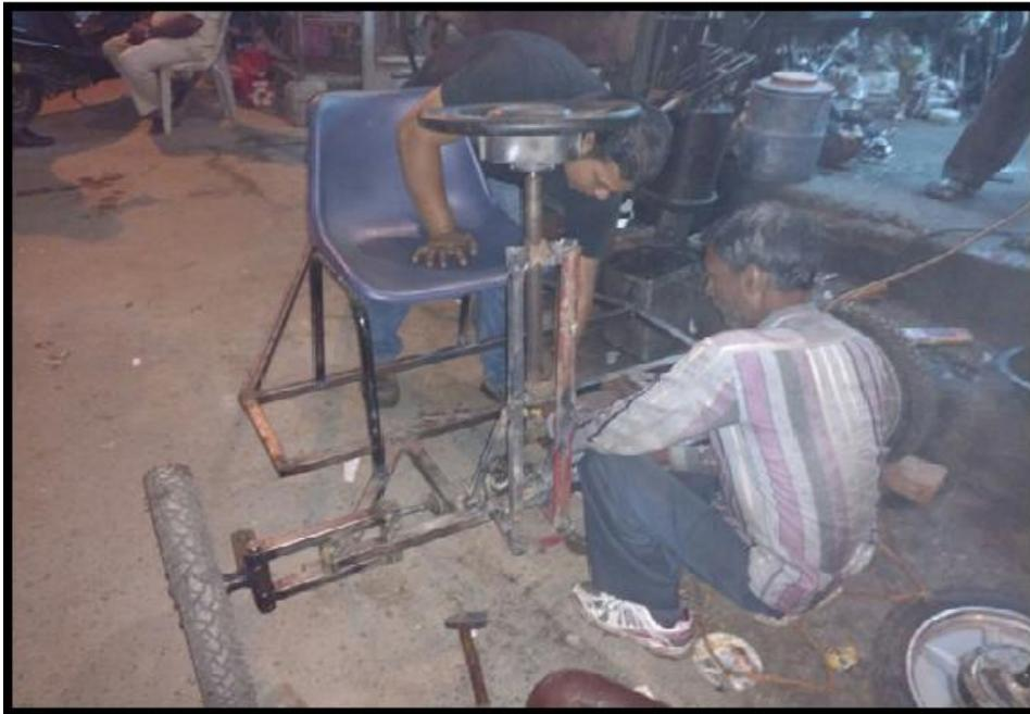
Figure: Workers helping in Adjusting Steering Column.
