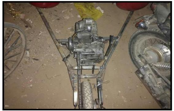
Figure: Entire view of the Transmission
