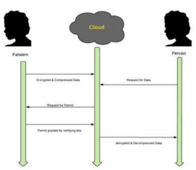
Figure 12. Sequence diagram of protected sharing.
