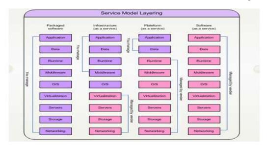
Figure 2. Service Model Layering 12.
