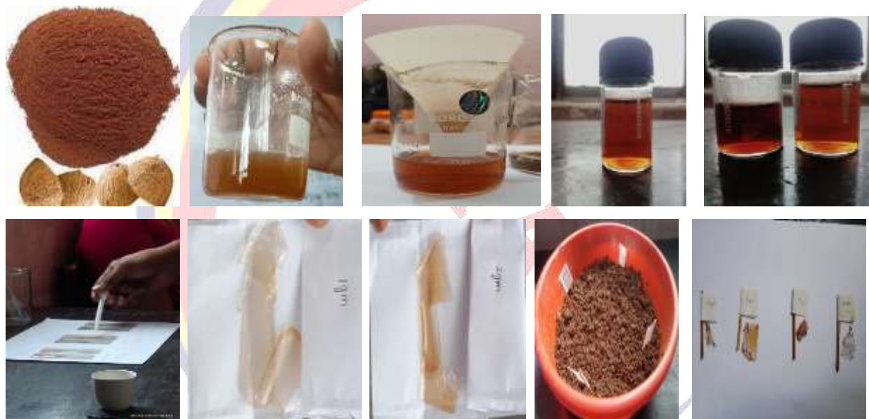
Fig 1. Preparation CSP solution in different Concentrations, films and buried in soil for biodegradation.
