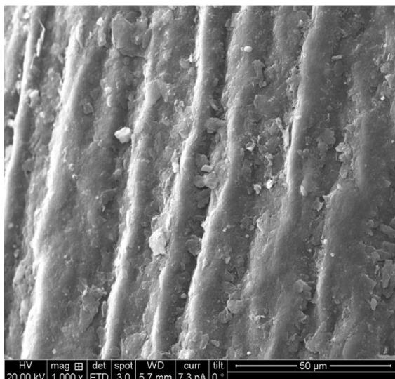
Fig.[3.3.8] Surface morphology (SEM) of 600°C (5 minutes) annealed red hot GR (0.25 mm) dipped in Nitric Acid (HNO<sub>3</sub>) solution (volume: 2.5 ml) for 30 seconds, shows shows an eagle view of perfectly aligned super matured vertical SWCNTs – tubular structure as closed individual fibres exhibit a middle hallow empty space (longitudinal view).
