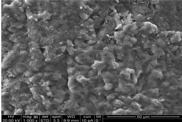
Fig.[3.3.5] Surface morphology (SEM) of 600°C (5 minutes) annealed red hot GR (0.25 mm) dipped in Sulphuric acid ( $H_2SO_4$ ) solution (volume: 2.5 ml) for 30 seconds shows imperfect, earliest growth, distribution, scattering and coagulation of hexagonal carbon matrices (basic building blocks of graphene layer) derived from core species.
