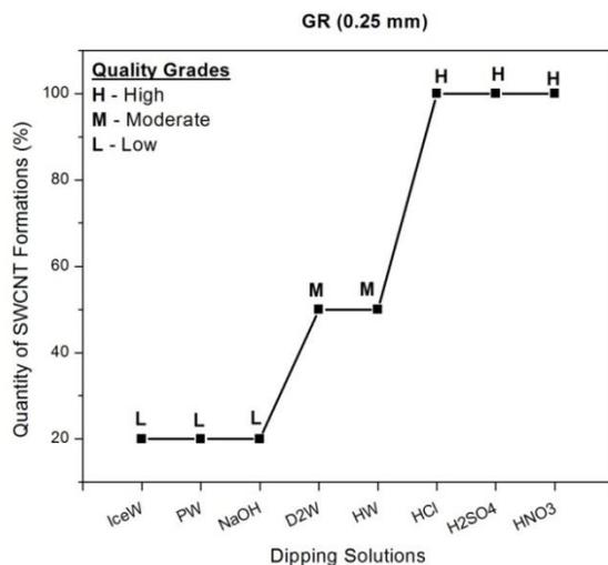
Fig. [4.1] Changes of Quantity of SWCNTs formation (%) with various Dipping solution with a note on Quality grades of developed SWCNTs from GR (0.25mm).
