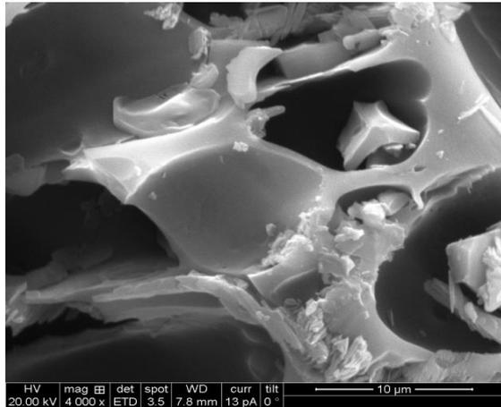
Fig.[3.3.3] Surface morphology (SEM) of 800°C (4 minutes) annealed red hot GR (0.25 mm) dipped in Hydrochloric acid (Hcl) solution (volume: 2 ml) for 45 seconds shows a damaged portion of the semi-matured stage of [eagle view] of vertical SW-CNTs. (cross-sectional view ).
