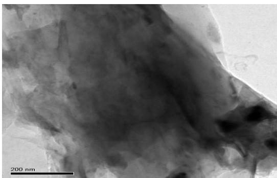
Fig.[3.4.3]. HRTEM image of un-matured intermediate stage of a graphene sheet from 600<sup>0</sup>C (1 minute) red-hot GR (0.25 mm) when dipping in Hydrochloric Acid (Hcl) (Volume: 1 ml) for 90 Sec.
