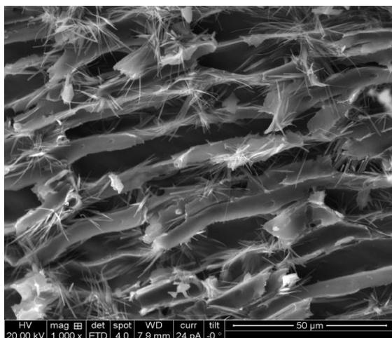
Fig.[3.3.4] Surface morphology (SEM) of 800°C (3 minutes) annealed red hot GR (0.25 mm) dipped in Hydrochloric acid (Hcl) solution (volume: 1.5 ml) for 60 seconds shows intermediate, damaged distribution of (tubular) rolled, scattered graphene layers belongs to horizontal SWCNTs (longitudinal cross sectional view). Due to poor coagulation, more star like patterns (composed of needle like grains) were obtained.
