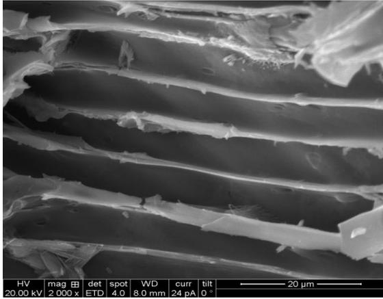
Fig.[3.3.1] Surface morphology (SEM) of 800°C (5 minute s) annealed red hot GR (0.25 mm) dipped in Hydrochloric acid (Hcl) solution (volume: 2.5 ml) for 30 seconds emphasized the clear evidence for the high grade super matured horizontal SWCNTs – perfectly aligned tubular structure of equal diameters (as rolled graphene layer which composed of hexagonal carbon matrix networks) (longitudinal cross sectional view) as individual fibres exhibit a middle hallow empty space (an eagle insight view).
