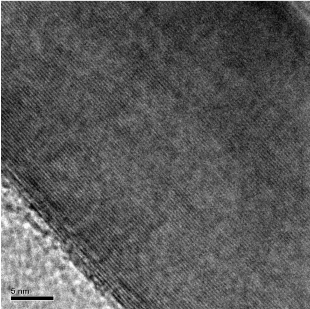
Fig.[3.4.2]. HRTEM image of super matured, perfectly aligned SWCNTs grown from 800<sup>0</sup>C (3 minutes) red-hot GR (0.25 mm) when dipping in Nitric Acid (HNO<sub>3</sub>) (Volume: 2.5 ml) for 30 Sec.
