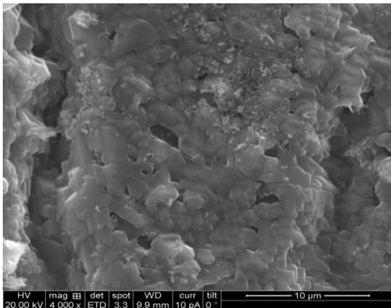
Fig.[3.3.6] Surface morphology (SEM) of 600°C (4 minutes) annealed red hot GR (0.25 mm) dipped in Sulphuric acid ( $H_2SO_4$ ) solution (volume: 2.0 ml) for 45 seconds, shows imperfect, just after initial budding growth, distribution, scattering and coagulation of hexagonal carbon matrices (basic building blocks of graphene layer).
