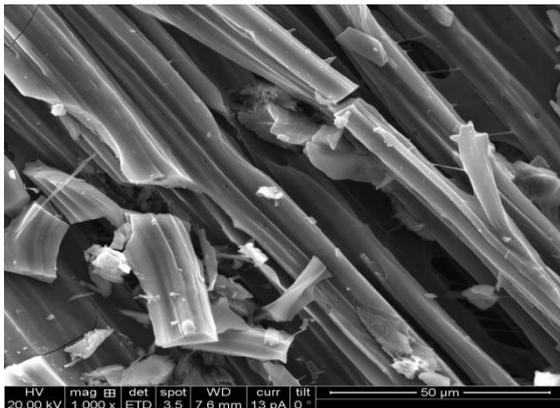
Fig.[3.3.2] Surface morphology (SEM) of 800°C (1 minute ) annealed red hot GR (0.25 mm) dipped in Hydrochloric acid (Hcl) solution (volume: 0.5 ml) for 120 seconds, shows very poor growth of damaged, inclined horizontal SWCNTs – tubular structure as closed individual fibres exhibit a middle hallow empty space (longitudinal cross sectional view).
