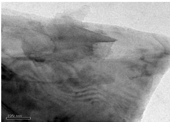
Fig.[3.4.6]. HRTEM image shows matured SWCNTs grown from 800<sup>0</sup>C (4 minutes) red-hot GR (0.25 mm) when dipping in Nitric Acid (HNO<sub>3</sub>) (Volume: 2 ml) for 60 Sec.
