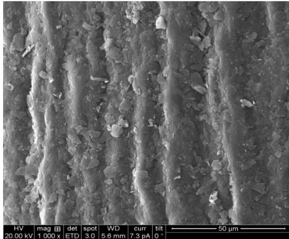
Fig.[3.3.7] Surface morphology (SEM) of 800°C (3 minutes) annealed red hot GR (0.25 mm) dipped in Nitric Acid (HNO<sub>3</sub>) solution (volume: 1.5 ml) for 45 seconds, shows an eagle view of perfectly aligned vertical SWCNTs – tubular structure as closed individual fibres exhibit a middle hallow empty space (longitudinal view).
