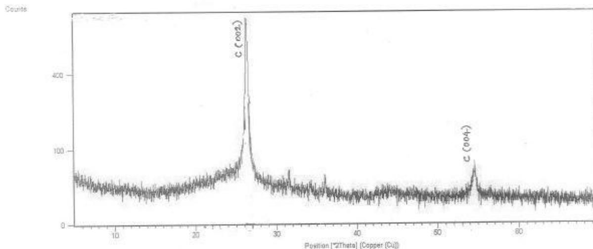
Fig. [3.1.1] XRD studies on GR (0.25 mm) annealed at 800°C (4 minutes) dipped in Hydrochloric acid (volume: 1 ml) for 120 seconds. The first order [C (002)] and second order [C (004)] diffraction peaks shows the single crystalline nature of the material.
