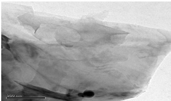
Fig.[3.4.5]. HRTEM image shows un- matured intermediate stage of SWCNTs grown from 800<sup>0</sup>C (2 minutes) red-hot GR (0.25 mm) when dipping in Nitric Acid (HNO<sub>3</sub>) (Volume: 2 ml) for 90 Sec
