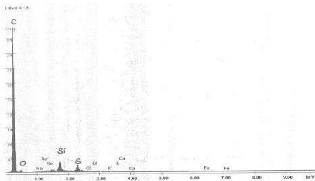
Fig. [3.2.1] EDAX studies on GR (0.25mm) annealed at 800°C (3 mints) dipped in double distilled water (DD water) (volume: 2.5 ml) for 30 seconds.
