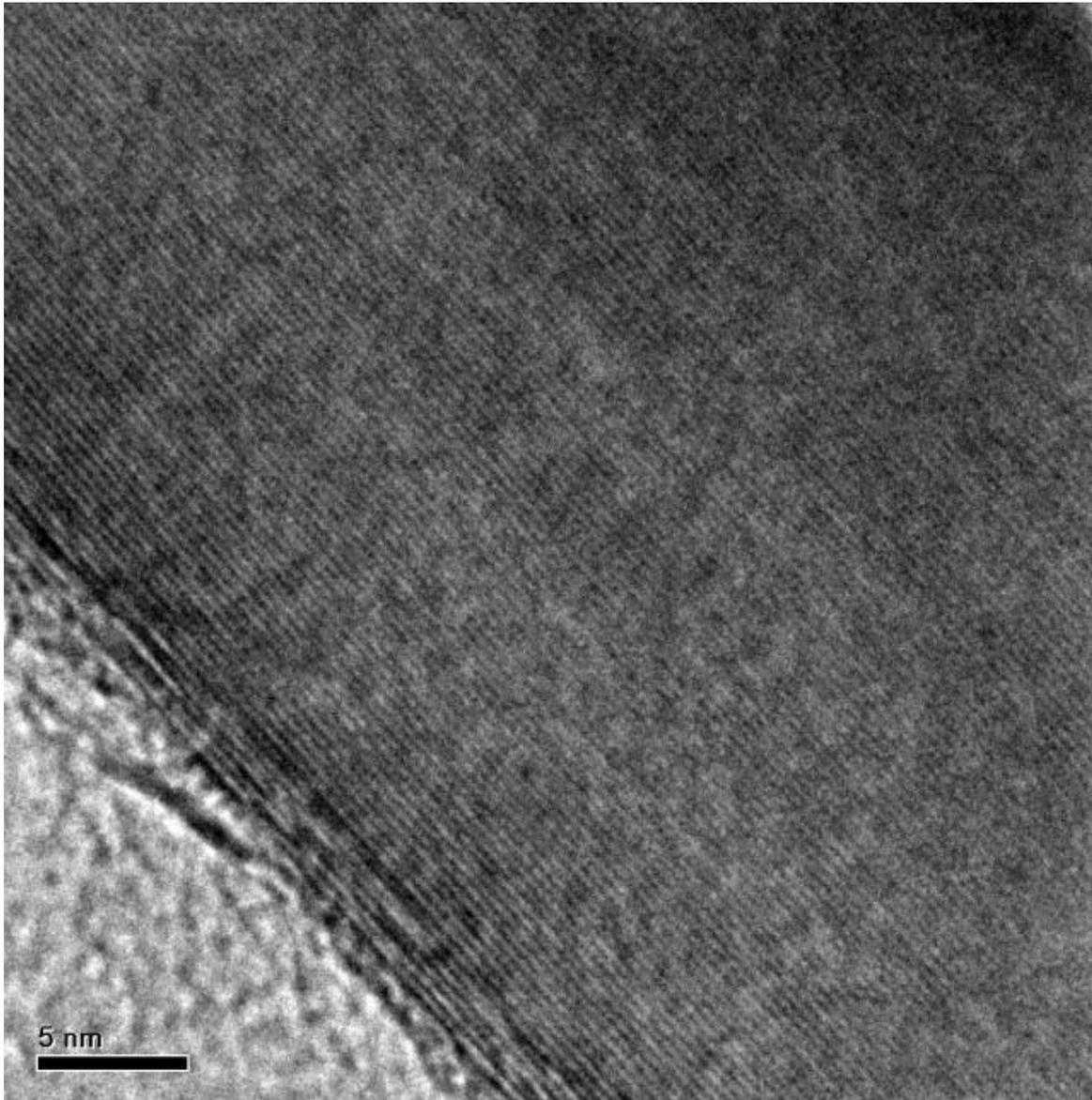
Fig.[3.4.1]. HRTEM image of super matured, perfectly aligned SWCNTs grown from 800<sup>0</sup>C (3 minutes) red-hot GR (0.25 mm) when dipping in Sulphuric Acid (H<sub>2</sub>SO<sub>4</sub>) (Volume: 2.5 ml) for 30 Sec.
