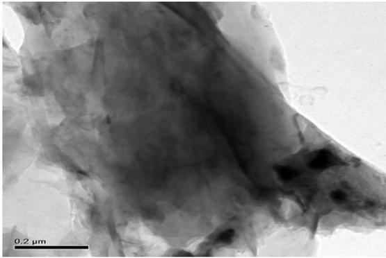
Fig.[3.4.4]. HRTEM image shows preliminary tubular formation of SWCNTs grown from 800<sup>0</sup>C (2 minutes) red-hot GR (0.25 mm) when dipping in Nitric Acid (HNO<sub>3</sub>) (Volume: 1.5 ml) for 120 Sec.
